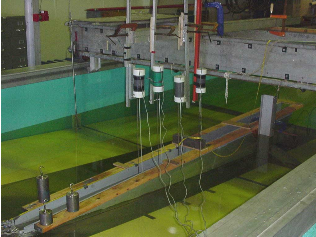
Figure 2: Quasi two-dimensional landslide experiments for benchmark case 2
