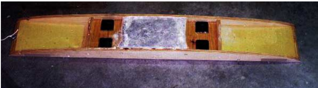
Figure 3: Close-up of scale model for two-dimensional landslide experiments
